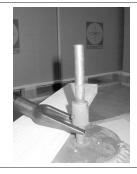
16.) Reassemble fan in reverse order. Apply a light coat of antiseize grease to motor plate, shaft extension and shaft.
