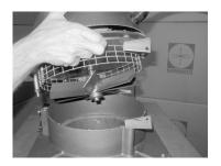
6.) Remove the 3 bolts holding the top cover onto the motor base and remove the top cover. Note the location of the motor wires and the top cover.
