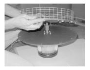
13.) Remove the motor mounting screws from the motor plate.
