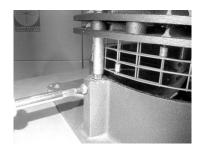
5.) Carefully remove the motor and fan assembly.
