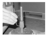
15.) RS 016 only: Using a pickle fork, leverage the shaft extension from the motor shaft.
