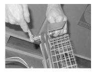
11.) Remove the front positioning bolt and spacer.
