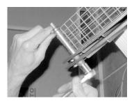
12.) Remove the cooling plate from the motor plate.
