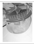
7.) Note location of fan on motor shaft. Using a 3 mm allen wrench, loosen the 2 set screws that hold the fan on the motor shaft.
