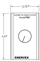
NOTE: The RSV and GSV 400 and 450 operate with 3-phase voltage and cannot be controlled with this kind of fan speed control.
